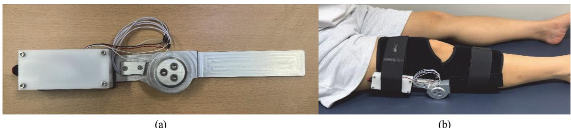
Fig. 2. (a) goniometer based on smartphone application; (b) wearable goniometer based on smartphone application.
